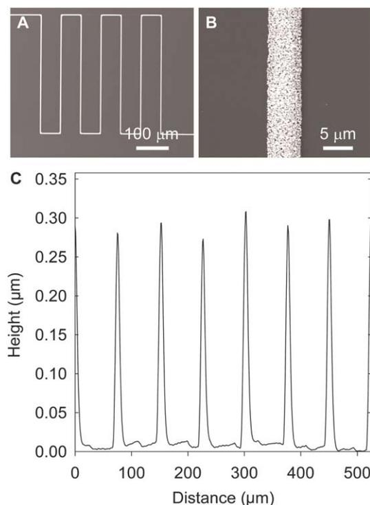
**Fig. 2** (A) SEM image of 1D serpentine pattern printed onto a silicon wafer with a center-to-center spacing between patterned features of 125  $\mu\text{m}$ . (B) Higher magnification SEM image of a conductive feature, and (C) height profile taken across the 1D array of patterned features.
