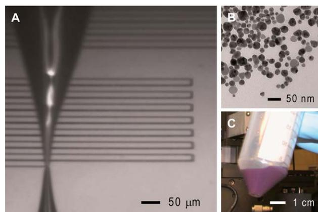
**Fig. 1** (A) Optical image of direct writing of silver nanoparticle ink on a silicon wafer using a 5  $\mu\text{m}$  nozzle. (B) TEM image of the synthesized silver nanoparticles. (C) Optical image of the concentrated silver nanoparticle ink (78 wt% solids).
