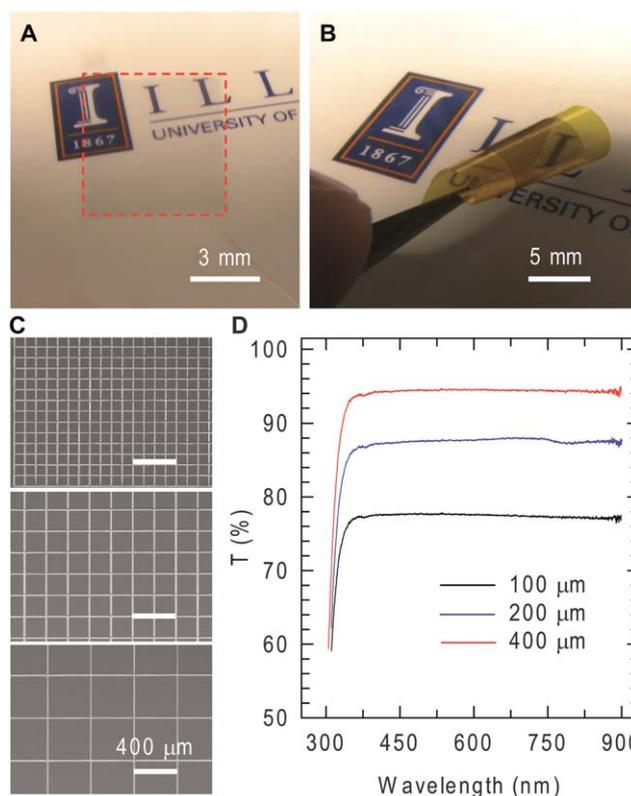
**Fig. 3** Optical images of the transparent conductive grids with center-to-center line spacing of 200  $\mu\text{m}$ , printed on (A) glass and (B) polyimide substrates. (C) SEM micrographs of the conductive grids, printed with center-to-center spacing of 100  $\mu\text{m}$  (top), 200  $\mu\text{m}$  (middle), and 400  $\mu\text{m}$ , respectively. (D) Transmittance of the conductive grids of varying center-to-center spacing patterned on glass substrates.
