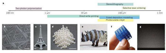
**Figure 2** | **Sizes and shapes of typical 3D-printed objects. a**, Coloured bars show the minimum size ranges of patterned features produced by several light- and ink-based printing methods. **b–g**, Examples of polymer constructs printed by: **b**, two-photon polymerization (hierarchical octet truss; scale bar, 25 μm; photo courtesy of J. Greer); **c**, continuous liquid interface production (Eiffel Tower; scale bar, 10 mm; adapted from ref. 27);
