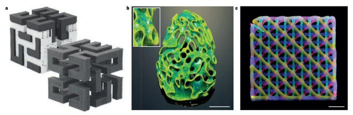
**Figure 3** | **Techniques for the fabrication of complex structures. a,** The white sacrificial support material in an FDM-printed part (back) is removed to reveal a Hilbert cube with numerous overhangs (front). (Photo courtesy of Polymaker.) **b,** A conceptual artwork by N. Oxman produced by multimaterial inkjet printing (scale bar, 10 cm). The inset shows the complex distribution
