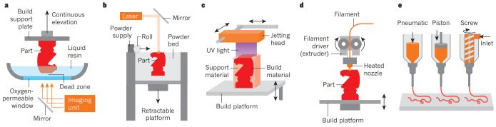
**Figure 1 Common light- and ink-based 3D printing methods. a**, The light-based 3D printing method known as continuous liquid interface production. (Diagram adapted from ref. 27.) **b**, Light-based selective laser
