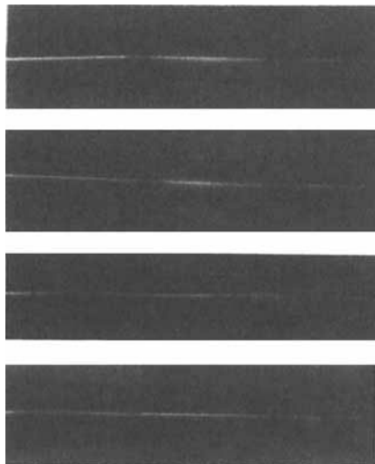
Fig. 2. Optical micrograph sequence of a PVB-DBP droplet inside a tapered glass capillary moving toward the narrow end of the capillary.
