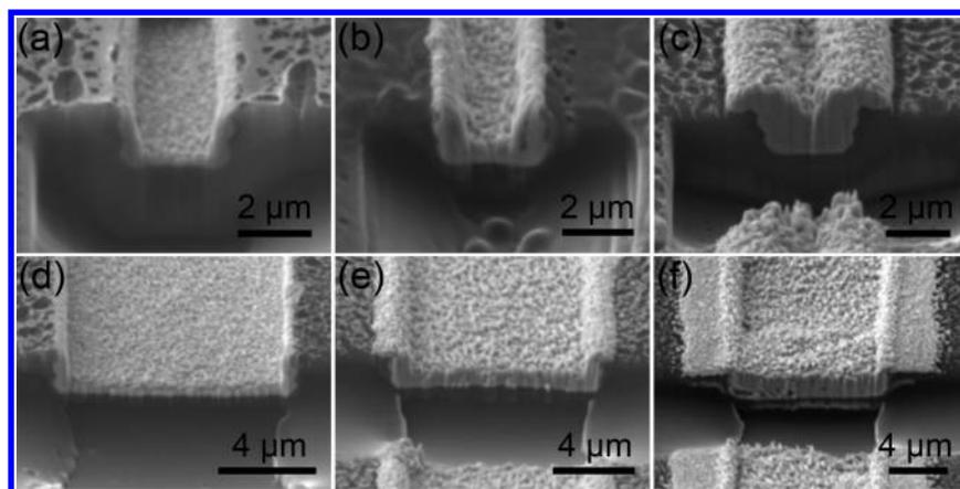
**Figure 3.** Electroless plating of Cu in printed microchannels. Focused ion beam cross sections showing Cu growth in a  $2.5\ \mu\text{m}$  wide channel after (a) 3 min, (b) 6 min, and (c) 9 min of immersion in the plating bath, and a  $10\ \mu\text{m}$  wide channel after (d) 3 min, (e) 6 min, and (f) 9 min of immersion. The depth of the channel in both the cases is  $2.5\ \mu\text{m}$ .
