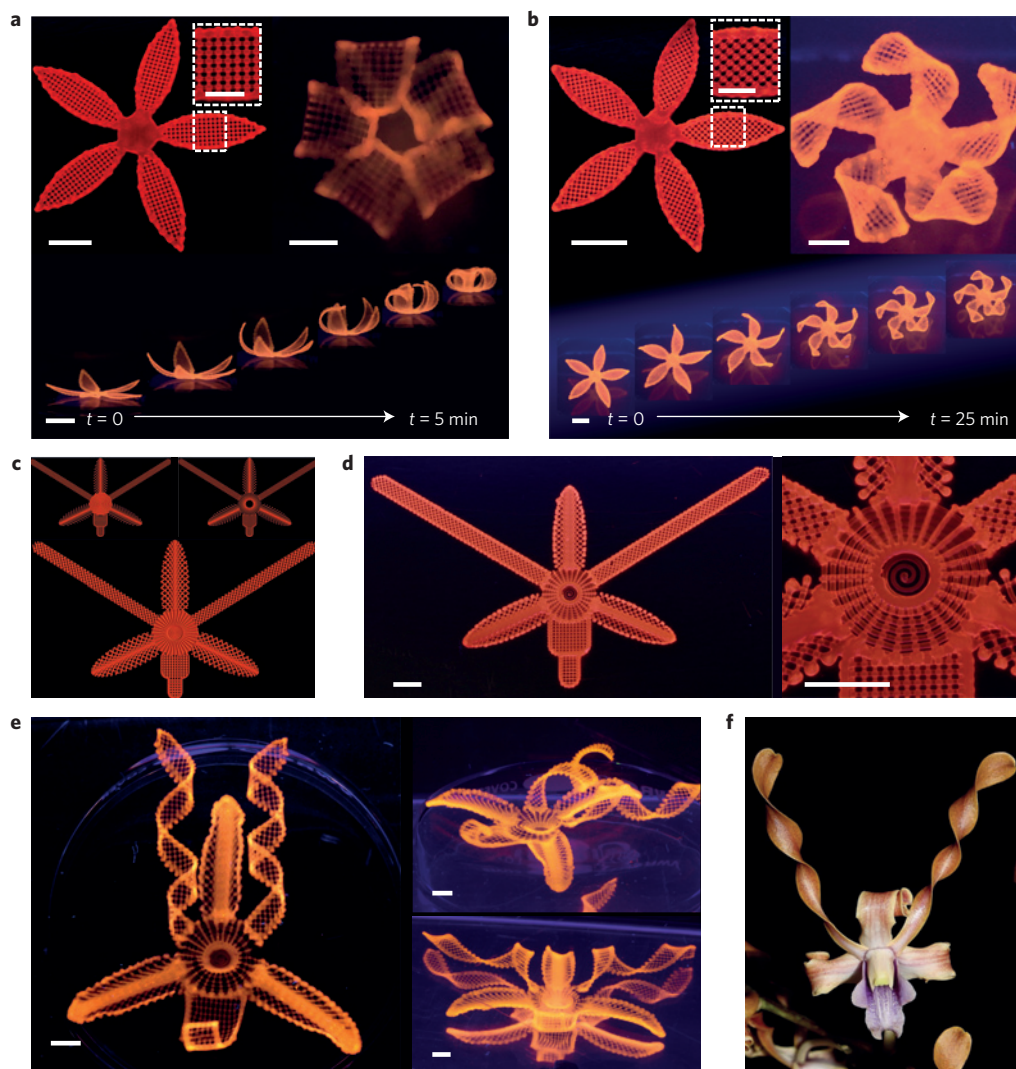
Figure 3 | Complex flower morphologies generated by biomimetic 4D printing. a,b , Simple flowers composed of 90^\circ/0^\circ ( a ) and -45^\circ/45^\circ ( b ) bilayers oriented with respect to the long axis of each petal, with time-lapse sequences of the flowers during the swelling process (bottom panel) (scale bars, 5 mm, inset = 2.5 mm). c-f , Print path ( c ), printed structure ( d ) and resulting swollen structure ( e ) of a flower demonstrating a range of morphologies inspired by a native orchid, the Dendrobium helix (courtesy of Ricardo Valentin) ( f ). Based on the print path, this orchid architecture exhibits four different configurations: bending, twisting and ruffling corolla surrounding the central funnel-like domain (scale bars, 5 mm).
